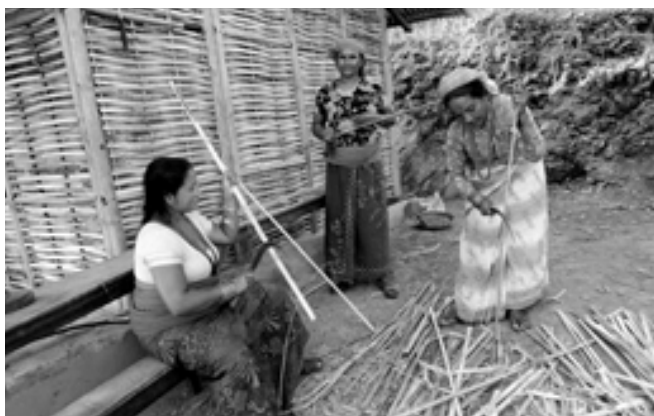
Women in Nepal prepare bamboo to be used as building material. In Jhapa, Habitat for Humanity Nepal has set up an enterprise to create corrugated roofing sheets out of bamboo mats. Women learn to produce the mats through a training program set up by Habitat Nepal.
